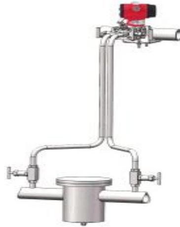
Pipe Differential Pressure Measurement
