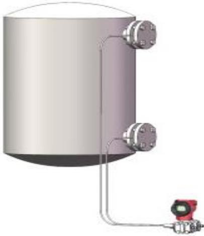
Tank Liquid Level Measurement
